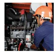
The machine has been designed keeping in mind the need to access key components with ease. The high clearance engine hood and full access side panels on both sides of the engine compartment gives easy access to the engine, flywheel and fan.
